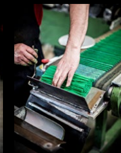
CARAN D'ACHE EXTRUSION OF LEADS
